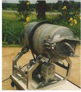
Fashioned from a 30-lb. propane tank, homemade parts "tumbler" takes the sharp edges off custom metalwork.
