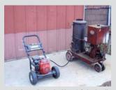
good shape. I plumbed in a 4-ft. hydraulic hose from the tank from the heater to the washer. Now I have 3,000 psi of hot water (approximately 150°) all for a few dollars. Works great to clean grease off equipment."
