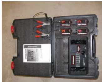
Road noise is transmitted to a headset connected to a receiver.
