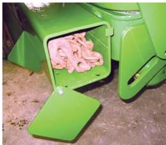
Front-end mounted chain box is made from 8-in. sq. tubing and has a cover at each end.
