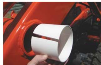
To cover a larger 4 1/4-in. dia. tube, he cut a slot in a 4-in. pvc connector fitting and slipped it inside tube. Expander plug fits into pvc fitting.
