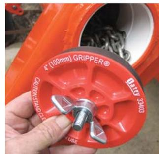
Dan Bodas stores chains, tools and pins in 4-in. dia. tubes on his Kubota tractor loader, covering the ends of the tubes with 4-in. dia. pvc expander plugs.
