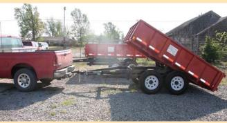
Operator sets the trailer brakes and then backs up. As upper frame and trailer box slides back past end of lower frame, it dumps.
