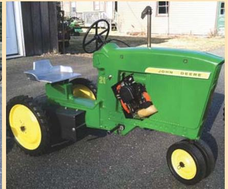
Tom Demers motorized this 1965 Deere Pedal Trac by installing an Echo 21 cc weed trimmer engine. It hooks up to a transmission off a Troy-Bilt mini rototiller, which chain-drives tractor's rear axle. Photo at left shows underside of tractor.
