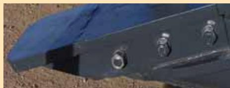
New replaceable knife tip has three release points.
