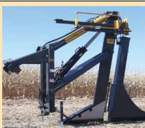
Interchangeable boots mount on quick-tach tile plow by simply pulling a single rod.
