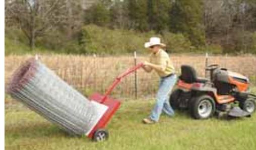
To load the wire roll, you grab a pair of handles at one end of tongue and pull it back toward the ground until the roll is in a vertical position.
