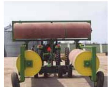
Side rollers pull straight behind raised center roller for transport.
