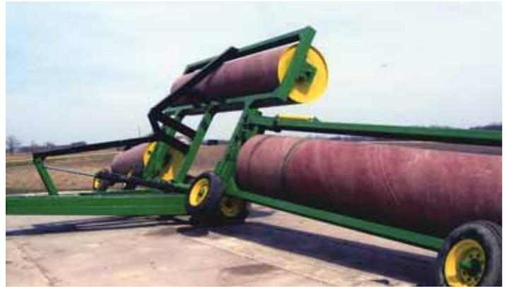
The cart that transplants the rollers is made from 2 used multi-weeder frames, welded one on top of the other.
