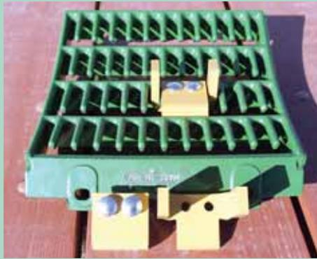
Disrupter lugs bolt to grates, (left). The lugs break up crop material in corn and beans. The new concave, (right), has 1/2-in. square keys instead of round bars, with 1 1/2 in. spacing between them.
