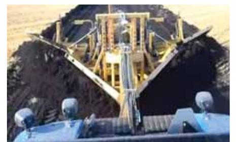
Heavy duty plow makes 32-ft. wide drainage ditches in a single pass. To see video on You-Tube search: V-wing ditcher, bigger, badder, faster!
