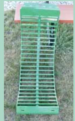
"The problem with the standard round bar concave in the Deere STS rotor is that there isn't enough space between the round bars to let grain out," says Estes. "We have designed a new grate that has 1/2-in. square keys installed instead of the round bars, with a 1 1/2-in. space between them for 68 percent greater openings."
