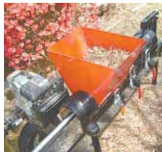
Splitter converts to a compressor with the addition of a hopper and compression chamber.
