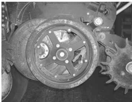
Open spoke design of new replacement gauge wheels keeps them free of mud.
