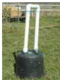
Photo shows closed loop of 2-in. dia. pvc pipe, which extends 8 ft. deep below ground (pipe loop in photo is just 4 ft. for demonstration purposes).
