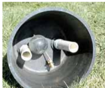
"Earth-heated" waterer consists of a 13-gal. plastic tub with pvc tubes and float assembly. Chickens drink through a hole cut into middle of tub's snap-on lid.
