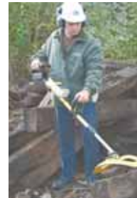
Handheld metal detector comes with a digital display screen and a head that tilts to any angle. It'll spot metal buried deep in logs.
