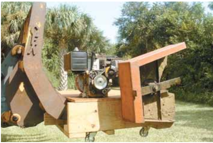
Home-built side cutter mounts on Combs' Case loader tractor and was built using part of an old Bush Hog mower and the motor from a pressure washer.
