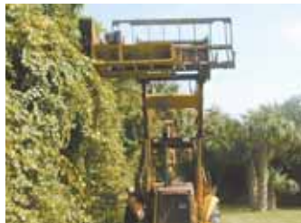
Combs can cut brush and vines in a 28-in. wide swath up to 12 ft. high.
