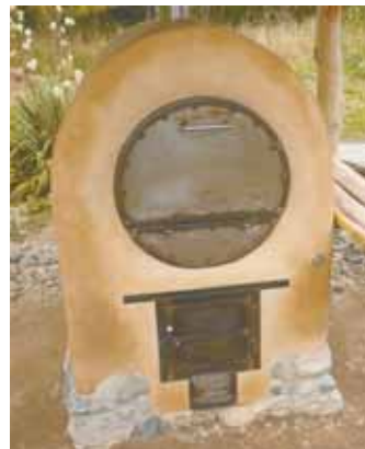
Barrel oven combines the best qualities of steel barrel stoves with traditional earthen or brick ovens. It has 2 racks and can bake up to 12 loaves of bread at a time.
