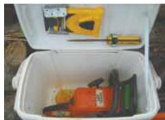
Brackets attached to bottom of cooler's lid are used to store other tools.
