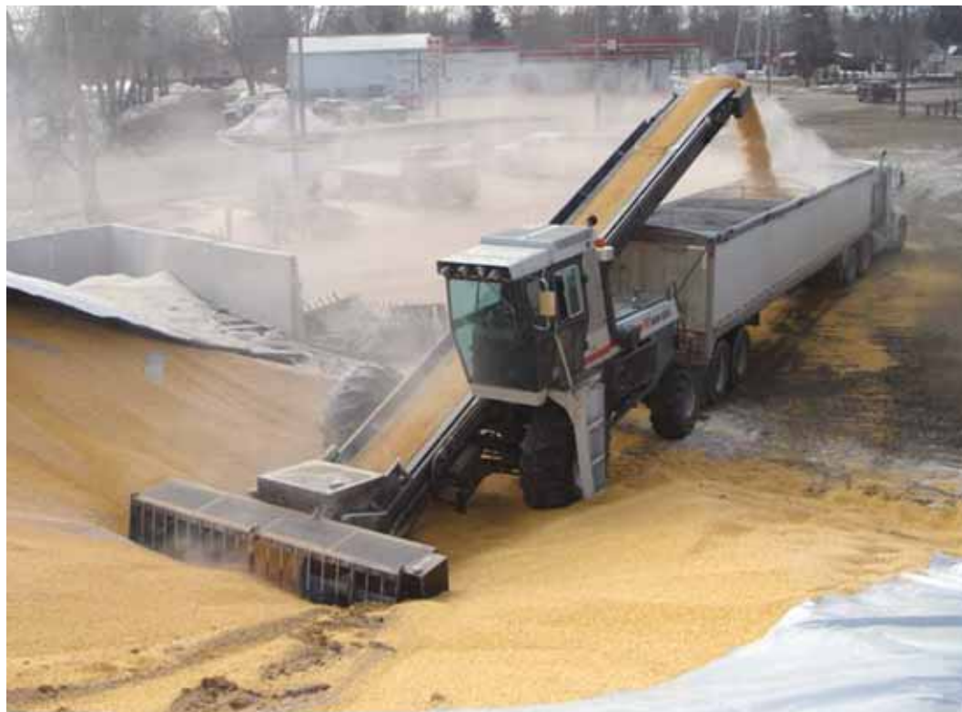
Swift "Gobbler" mounts on a Uni Harvester and is designed to load 20,000 bu. of grain per hour. It features a 12-ft. wide detachable auger header and a 50-ft. long by 3-ft. wide high speed conveyor belt.
