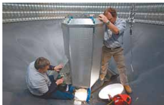
"Retro Rocket" aeration kit can be used in existing hopper bottom bins. It reduces grain drying time and increases fan efficiency by forcing air into center of bin.
