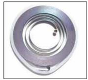
winding it tightly enough to fit back into its housing. Here's how to solve the problem. Pound a nail into the center of a small piece of plywood and attach the outer edge of the recoil spring to the nail, then attach a drill to the inside edge of the spring. As you begin to slowly advance the drill, the spring will wind and tighten. You may have to hold your hand flat over the spring while winding to prevent it from flying apart.
