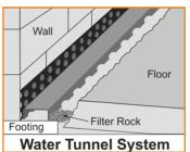
The Water Tunnel System is installed on top of the footing. Helps relieve hydrostatic pressure from the walls and under the floor. Less concrete and dirt is removed, drastically cutting installation costs, compared to conventional drain tile systems. The easy to install system, collects the water from the walls and under the floor footing area, channeling it to a sump pump.
