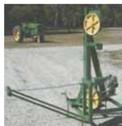
Bandsaw is belt-driven by a 3 hp., Briggs and Stratton engine.
