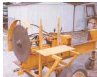
"I can quickly cut up smaller logs and branches with the saw and run bigger logs through the splitter," says Harold Schenk about his home-built splitter-saw.
