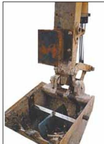
A 4-way cutter mounts inside backhoe bucket and a block of I-beam mounts on boom. To split wood, Forester places a chunk on top of cutter and retracts bucket's hydraulic cylinder.
