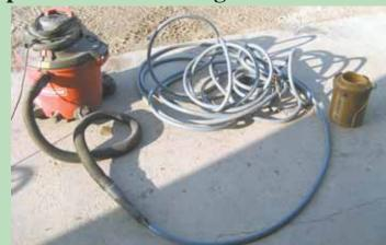
Roger Gutschmidt used a shop vac to suck baler twine through a length of flexible conduit, then tied the twine to electrical wire to pull it through.
