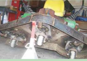
Front-mount mower deck is designed with the caster wheels underneath the deck – rather than out front – and new-style mower blades that rotate around them.
