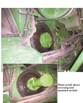
Special hub fits over the pulley of combine's discharge beater, allowing you to use Deere's reversing tool to clean out a plugged beater.
