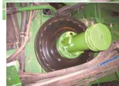
**Photo at left shows reversing tool mounted on hub.**
