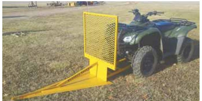
**You can quickly cut trees with an ATV using Hav-Roc's new "mini" model. V-shaped design has teeth that work like a big handsaw.**
