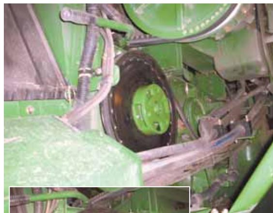
**Special hub fits over the pulley of combine's discharge beater, allowing you to use Deere's reversing tool to clean out a plugged beater.**
