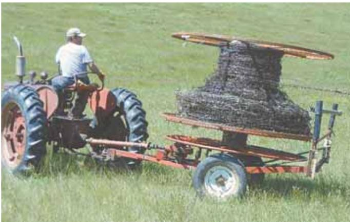
**Big 7-ft. dia. reel mounts on an old pto-powered irrigation hose winder. It can wrap up miles of 3-strand fence wire at a time.**
