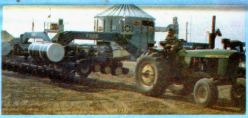
New swinging toolbar allows you to carry fertilizer or no-till attachments on the planter, plus up to 49 row units (for soybeans) without overloading the toolbar and without restricting its ability to swing to less than 13 ft. wide for transport.
