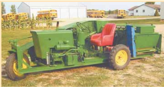
The operator rides in comfort on a cushioned chair while steering a single front wheel. Foot and hydraulic controls are within easy reach.
