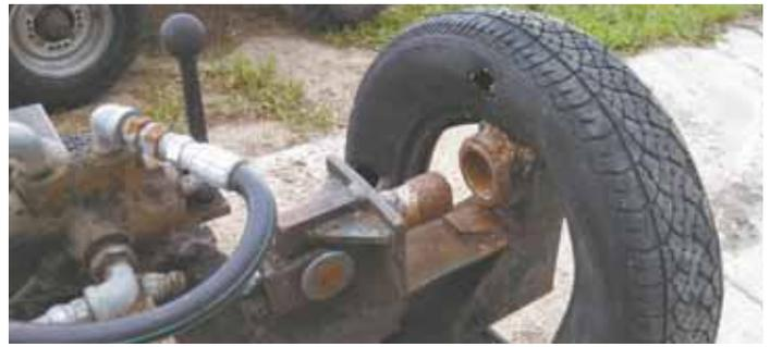
A hydraulic-operated, 3-in. dia. rod is used to punch holes through the rubber.
