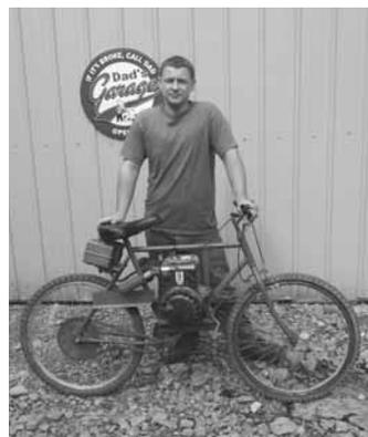
Glenn Sherwood built this motorized bicycle that's powered by an old 8 hp Tecumseh engine. It belt and chain-drives the bike's rear wheel.
