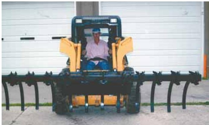
Old chisel plows can be converted into heavy-duty brush rakes. "They work great to handle cut-down cedar trees and brush," says Perry Easley.
