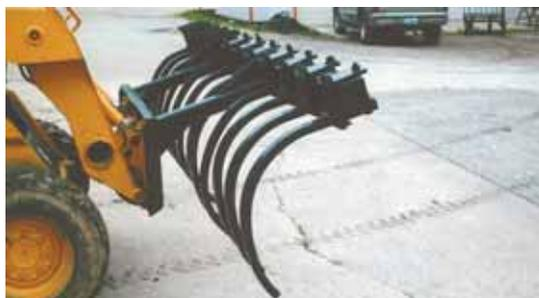
He welded his 10-ft. rake to a quick-tach hook-up on his skid loader. Shanks are evenly spaced about 1 ft. apart.
