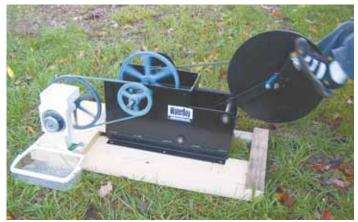
Pedal-powered pto work station can be used to operate any low rpm tool, including alternators, grain grinders and even power shop tools.
