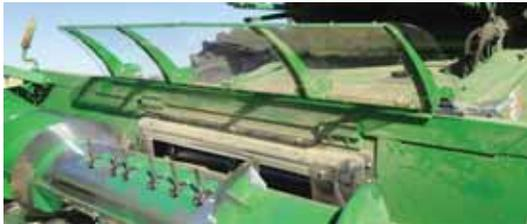
Scratch-resistant clear Lexan shield blocks kernels from being thrown out of header.
