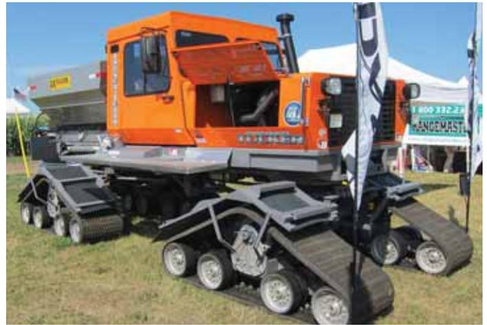
Ag Tucker Terra rides on 4 steerable tracks and comes with a 3-ton granular fertilizer tank and spinner spreaders, or a 500-gal. spray tank with booms up to 90 ft. long.
