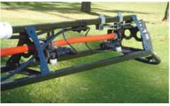
**GPS-guided spraying** system turns spray nozzles on or off individually to virtually eliminate over and under
