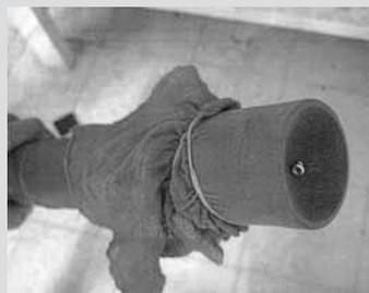
**Joe Williams, Maple Grove, Minn.:** “If you drop a ring, a bolt, or other small part down a sink drain, you can get it out easily without having to get out your plumbing tools. Just stretch a nylon stocking over the nozzle of a shop vac and stick it over the drain. Whatever it pulls up will stick to the nylon for easy retrieval.”
