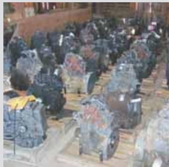
Japanese New Holland engines, often called JSM or Shibaura engines. They’re found in compact Ford New Holland tractors and skid loaders. Weavers sells new aftermarket piston rings, bearings, and gaskets for these engines and also sells used and/or reconditioned blocks, cranks, rods, heads, etc. They also have new overhaul kits starting at \$595 complete, as well as rebuilt engines.
