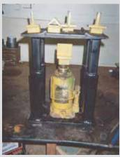
Harold Fratzke, Cottonwood, Minn.: "I made a portable hydraulic press that can be used with any hydraulic jack.
