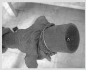
Joe Williams, Maple Grove, Minn.: "If you drop a ring, a bolt, or other small part down a sink drain, you can get it out easily without having to get out your plumbing tools. Just stretch a nylon stocking over the nozzle of a shop vac and stick it over the drain. Whatever it pulls up will stick to the nylon for easy retrieval."
