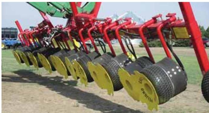
Update kit uses notched metal discs that bolt on in pairs on back of rubber wheels. One disc is flat and the other one is curved and faces backward. The curved disc is bigger than the rubber wheel, so the two discs overlap each other by half an inch.
