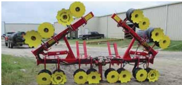
Machine's rubber wheels and rollers grab the weed, and then the weed gets caught in the notches between the 2 discs and pops out of the ground.
