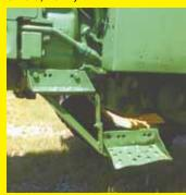
Due to health issues, I needed to reduce the height of the first step on my Deere 3020 tractor. I moved the right hand step, which was never used, to the left side. Using some flat iron, 4 bolts, and welding an angle brace, I was able to reduce that first step by 8 in. The ground to first step is now 17 vs. 25 in. The same idea can be used on a 4020. (Ron Roberts, 1518 S. Prairie Rd., Stillwater, Okla. 74074, ph 580 371-5333).
