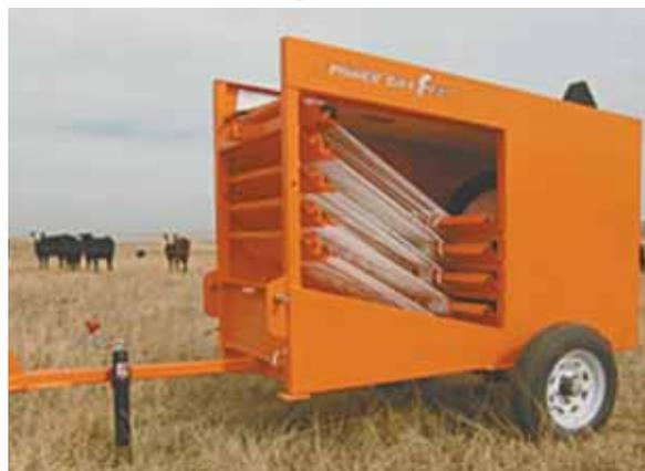
Power Grazer portable fencing system makes putting up temporary fencing a quick and easy job.
