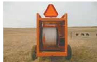
Solar-powered batteries operate a reel that winds up fence.
