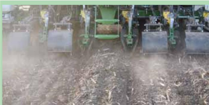
Planter-mounted tillage system eliminates soil compaction in wheel tracks caused by the planter and tractor during planting.
