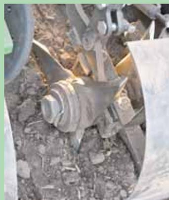
Three 9-in. tines per hub shatter the soil to allow water to soak in.
