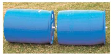
Barrels are strung together by lengths of pvc pipe and sealed with silicone to stay watertight.
