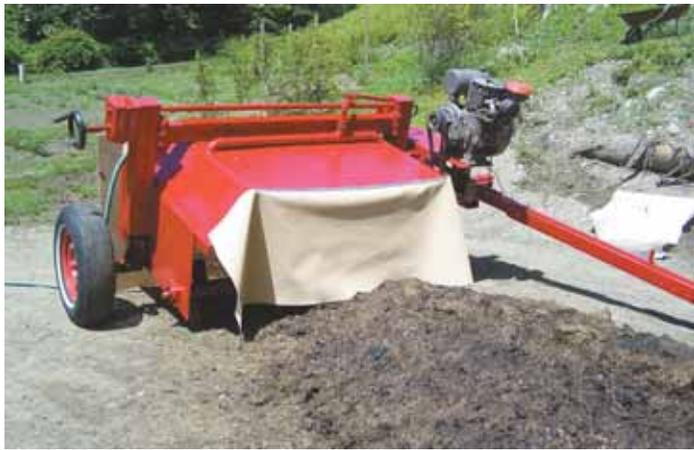
Russell Wing spent less than \$300 to build this pull-type compost turner that's powered by an old Wisconsin engine.
