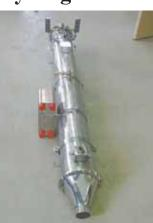
Heat Collar channels exhaust through a pipe filled with small tubes, capturing otherwise wasted heat from stationary engine exhausts.
