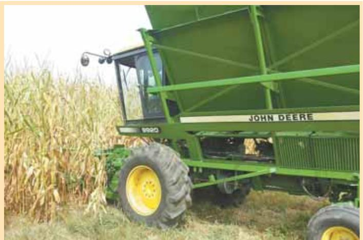
**To improve visibility, he lowered the cab by about 6 in. The cotton basket was replaced by a side-dump box from a silage wagon.**
