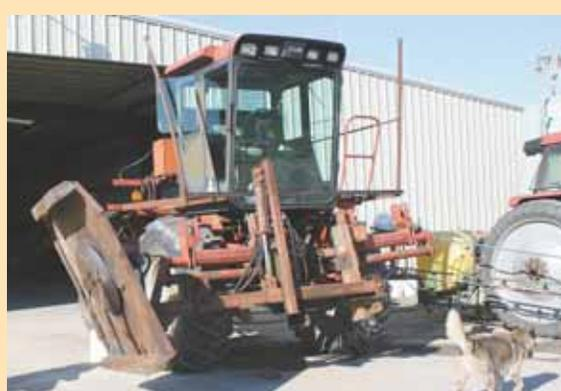
**To build this ditch bank mower, James Doughtie stripped all cotton components off an old cotton picker and then mounted a 3-pt. mounted deck mower on the header pickup arms.**
