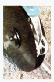
The 3½ in. dia. wheel scrapers turn as the disk they rub against turns. They can be replaced in seconds without having to dismantle the disk assembly.
