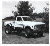
fitted with 36-in. tires. He installed a 4-in. high suspension system and raised the body another 2 in. The Chevrolet "big block" 402 cu. in. gas engine came from a 1971 pickup, and the automatic transmission with overdrive was taken from a 1984 Chevrolet Blazer.
