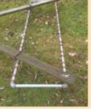
Roland Erikson pulls this 74-in. wide rake behind his riding mower to remove debris from his yard. Rake's 24 tines attach to 2 galvanized water pipes.
