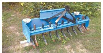
Dex Brouillette converted a standard 6-ft. box blade into this heavy-duty unit equipped with 11 rippers.
