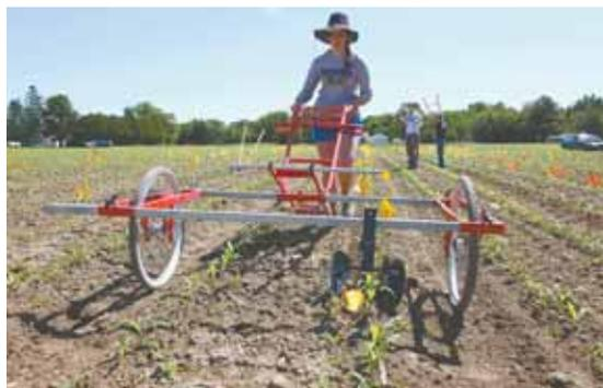
Weed Master's parallel linkage design makes it easy to use a variety of tillage tools, such as this tiller attachment.
