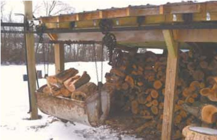
Tracked manure carrier brings wood from a shed to Norenberg's outdoor furnace. To mount the track, he extended the eave on his woodshed and mounted the rail beneath it.
