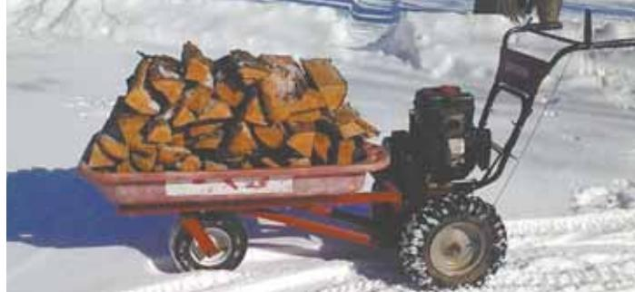
Bledsoe unbolted the blower and auger from a walk-behind snowblower and mounted a small wagon box in their place. It rides on a single caster wheel.
