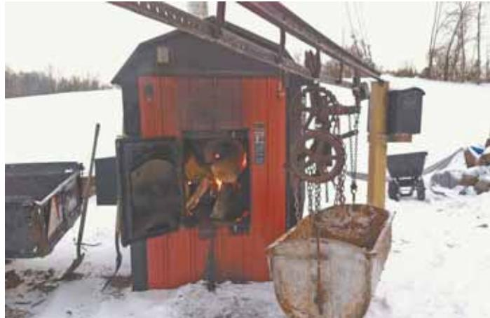
A chain hoist is used to raise and lower the carrier for easy loading and unloading.
