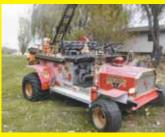
A friend of mine gave me a Kawasaki Mule that had burned up in a garage fire. The only salvageable part was the drive axle so I cut off the frame right ahead of the axle and then started building a miniature fire truck. Kids love it. Comes complete with a ladder, flashing lights, and a siren
