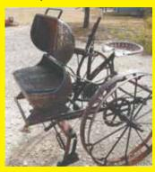
I built a barbeque grill out of an antique seeder with a propane tank mounted on front. I cut the tank open and installed a handle, hinges, and a grill. It looks pretty nifty and we can roll it around to wherever we want to use it. (Joel Lawler, 282 PR 265, Bowie, Texas 76230 hillbilly265@att.net)
