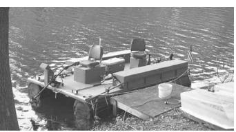
A pickup ladder rack forms the frame of this "fishing boat" pontoon built by Robert John. It floats on six 55-gal. plastic barrels and has two 12-volt trolling motors.
