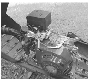
gas runs through hoses into the tractor's engine, a 6 1/2 hp. Honda clone. fabricated carburetor to better match the engine to the charcoal gas output.
