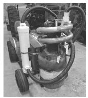
Pvc "filter" pipes are connected in series, mounted on each side of the tractor.
