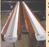
Hall frames gutters with end caps and plastic floats inside treated 2 by 4's. A 3 in. net cup at bottom of bucket allows water to be drawn up into potting mix.
